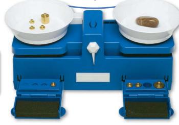
Add gram masses to the other pan until the two pans are balanced. Then add the values of the gram masses to find the total mass.
